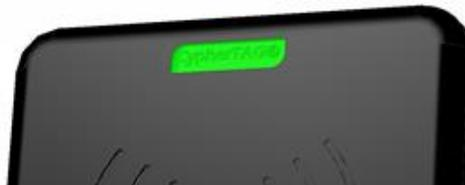
3. The RELV1 sends the identity of the tag once when the tag is first identified. To get another report, take the tag away from the RELV1 for the duration of the tag timeout (refer to the configuration sheet) and then present the tag to the reader.
