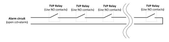
Series connected, using normally open contacts that close in correct operation
